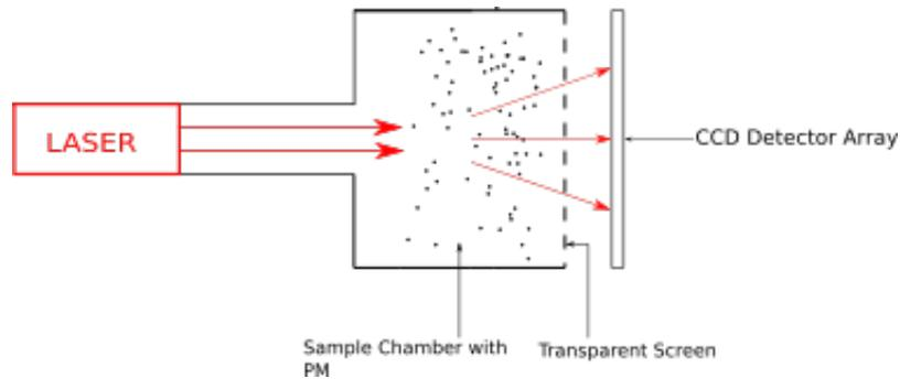
FIG. 1. Schematic of a typical aerosol counter
