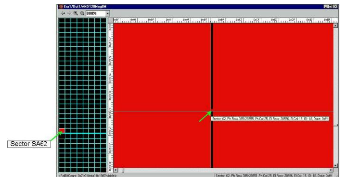
Figure 15: Bitmapping results using a memory tester showed a leaky column (unable to be programmed) and a leaky row at the failing sector. The arrow pointed to the intersect cell which was suspected to be the cause for the failing row and column.
