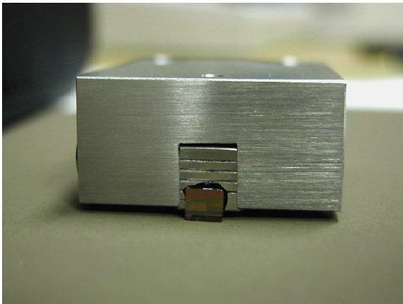
FIGURE 7b: Alternate view of polishing block with illustrative sample mounted.
