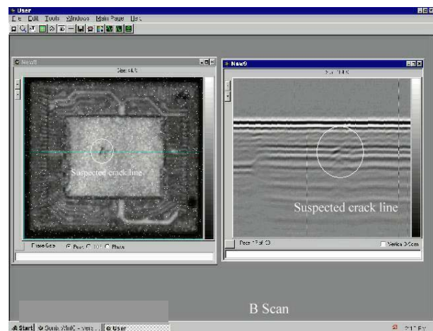
Figure 12: SAM C-scan (left) and B-scan (right) results showed a possible die crack at the failing sectors location (circled)
