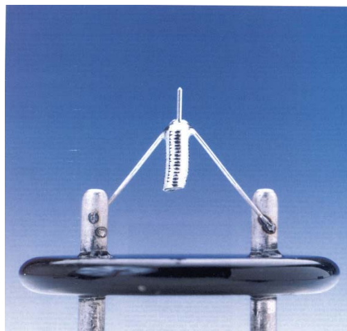
Figure 1: Actual gallium LMIS used in contemporary FIB systems, consisting of a W tip and a reservoir mounted on a metal/ceramic substrate. Ceramic diameter ~ 1cm.
