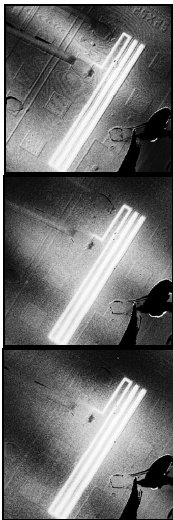
Figure 27 - Fluorescent microthermal images illustrating the reduction in spatial features after UV film stabilization (top to bottom: t = 20 \text{ sec} , t = 600 \text{ sec} , t = 1200 \text{ sec} ).
