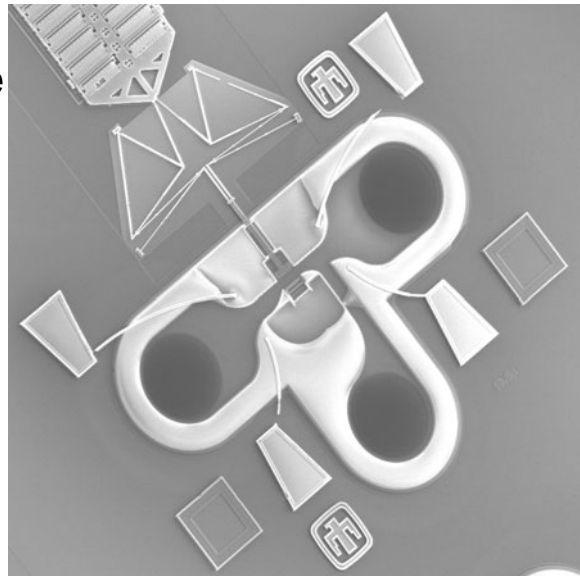
Fig. 1. a) bulk micromachining process illustrates patterning through the bulk material to fabricate a MEMS device. b) bulk micromachined device with surface micromachined top layers form a fluid transport manipulator capable of processing various materials in a fluidic medium.
