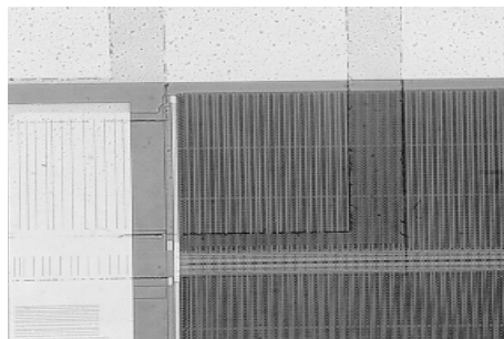
Figure34. Image of the device ready for Metal 3 removal.
