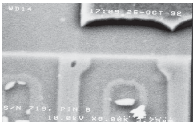
Figure 16 - Typical customer return showing a single small hole in the gate oxide.
