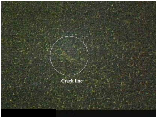
Figure 13: Re-examination on the FBGA package surface showed a faint crack line at the suspected area (circled)
