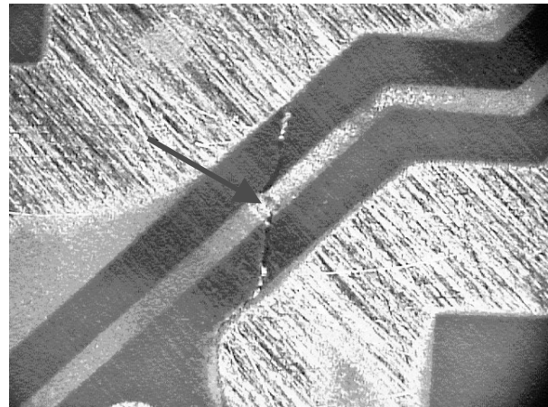
Figure 18. Optical image showing a broken trace in the package substrate
