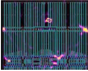
Figure 10: Backside current image of a standby current failure on a SRAM. The defect is indicated by the arrow and the whole image is overlaid on a CAD layout.
