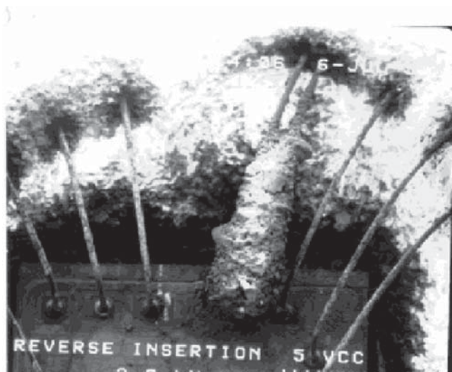
Figure 18 - Carbonized plastic surrounding the Vcc dual bond wires and adhering to the die surface of a PDIP packaged device.
