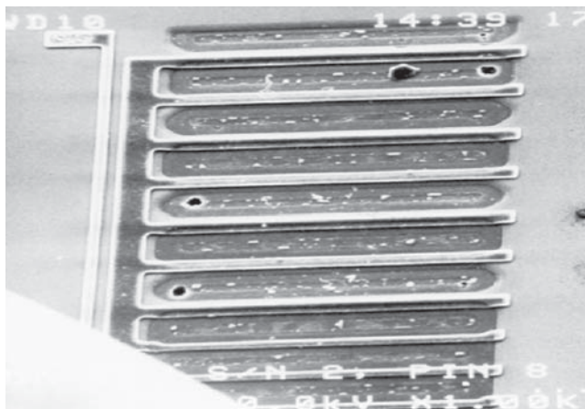
Figure 8 - MM. Severe damage at the contacts of the ESD protection structure.
