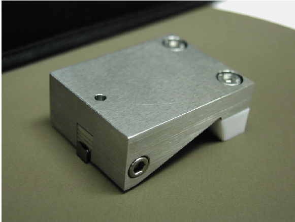
FIGURE 7a: Overall view of polishing block with illustrative sample mounted. The side screws hold the removable stud in. The adjustable Teflon heel is seen on the other end.
