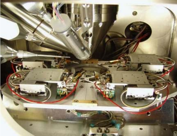
Fig. 13: 4-probe nanoprobe, mounted on a stage of a Dualbeam FIB.
