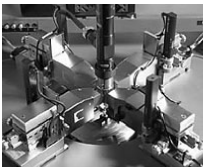
Figure 30: AFP probe tips showing the probe entrant angle. Courtesy Multiprobe Inc.
