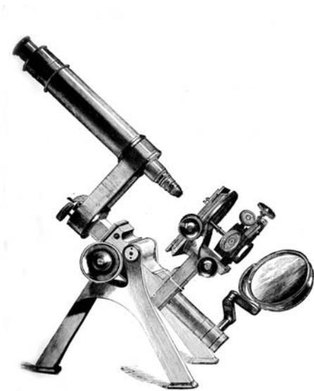
Figure 2: A simple 1920's microscope showing eyepiece, tube, objective, sample stage and illumination source. From Spitta, 3 rd edition [1].
