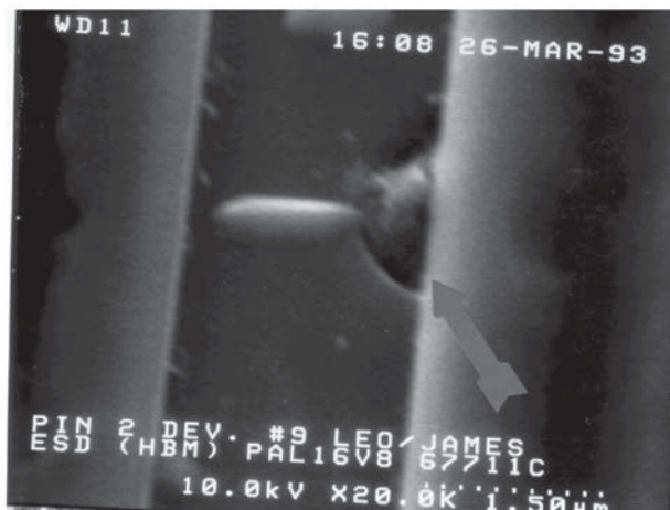
Figure 4 - Subsurface ESD damage to the contact at the failure site in the ESD protection circuit. There is no discoloration.
