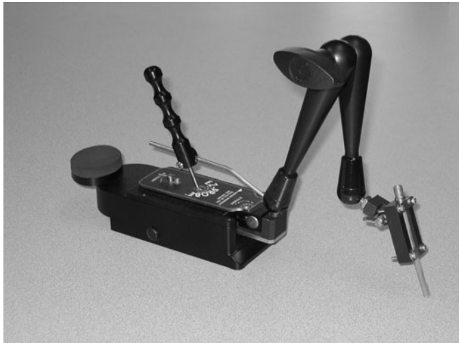
Figure 13. TDA Systems QuickTDR™ probe supported by Cascade Microtech EZProbe™ positioner. The spacing between signal and ground in the tip of the probe is extremely small to ensure best performance
